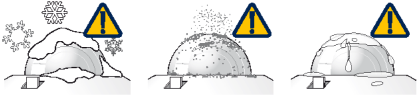
FIGURE 8-1. Reading is reduced if dome is not dry or clean
